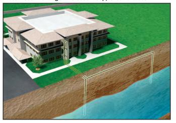
• Closed Loop/Ground Water Plate Heat Exchanger Systems utilize lake, ocean, well water or other water sources to maintain closed loop water temperatures in multi-unit large water-to-air systems. A plate frame heal exchanger isolates the units from any contaminating effects of the water source, and allows periodic cleaning of the heat exchanger during off peak hours.
