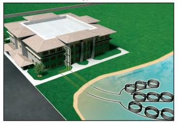
• Closed Loop/Ground-Source Surface Water Systems also utilize the stable temperatures of Surface Water to maintain proper water source temperatures for large water-to-air units extended range heat pump systems. These systems have all of the advantages of horizontal and vertical closed loop systems. Due to the extended loop temperatures, AHRI/ISO 13256-1 Ground Water or Ground Loop Heat Pumps are required for this application.
