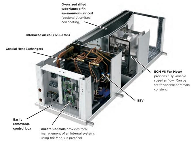
Four blower discharge options are available. Factory or field conversion option of end or side discharge using switchable access panels and a factory only option of true left or right return air coil.
