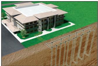
• Closed Loop/Ground-Source Systems utilize the stable temperatures of the earth to maintain proper water source temperatures (via vertical or horizontal closed loop heat exchangers) for large water-to-air units extended range heat pump system. Sizes range from a single unit through many hundreds of units. When net cooling requirements cause closed loop water temperatures to
