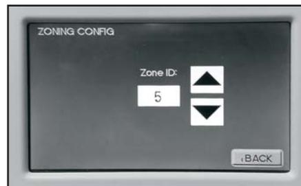
Use the up/down arrows ▲▼ to select the zone. If more than one zone is assigned the same zone number an error will be displayed on the TPCC32U01 and MasterStat. After the initial configuration, to change the zone numbers enter the configuration mode by holding a finger over the Zone number in the upper left hand corner of the Main screen for 5 sec. Select zone number and use the up/down arrow ▲▼ to adjust.
