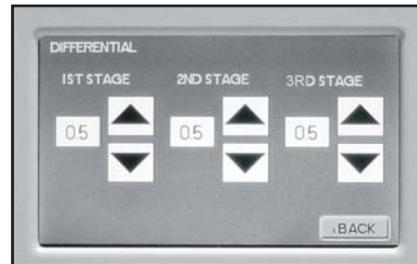
This adjustment will vary the number of degrees, from the set point, before a call for heating or cooling is made. Adjustments can range between 0.2° and 4° differential. Default is 0.5° differential. (If your set point is 70° in heating, your thermostat will not call for heat until the room temperature is 69.5°, when using a 0.5° differential setting).
