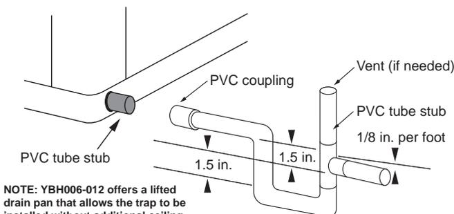
NOTE: YBH006-012 offers a lifted drain pan that allows the trap to be installed without additional ceiling height required.
