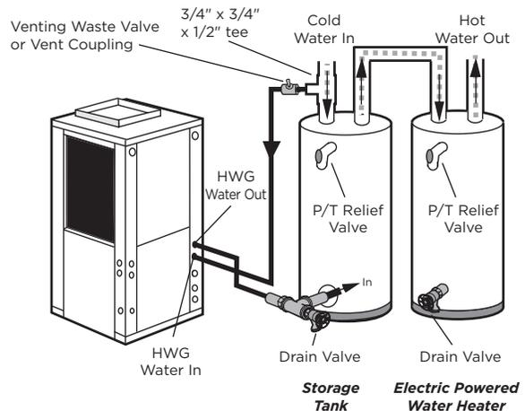
**NOTE:** This configuration maximizes hot water generator capability.
