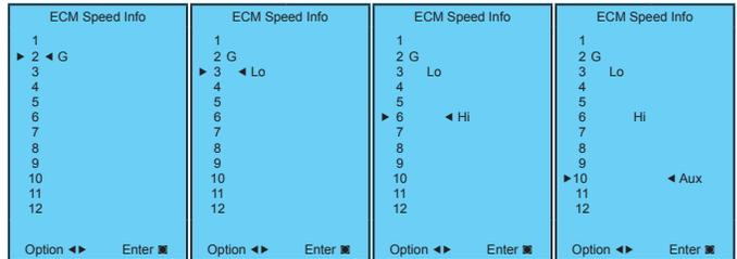
After the auxiliary heat speed setting is selected the AID Tool will automatically transfer back to the ECM Setup screen.
