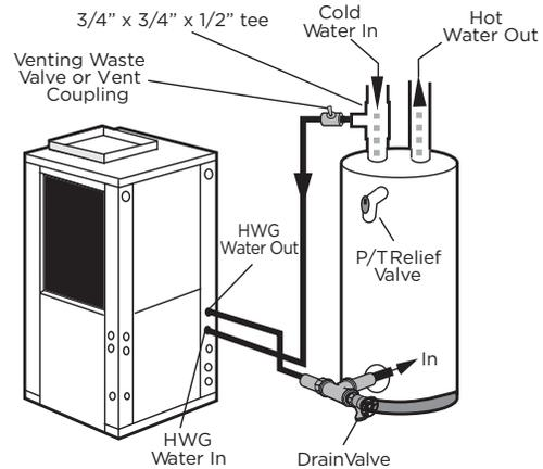
**Figure 12: Hot Water Generator Installation In Preheat Tank**
