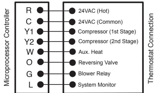
**Figure 22: Thermostat Wiring (Communicating Style Signals)**
