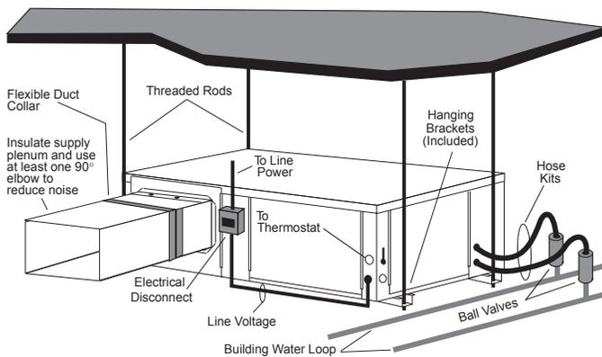
in Figure 3. The unit should be pitched approximately 1/4-inch towards the drain in both directions to facilitate the removal of condensate. Use only the bolts provided in the kit to attach hanger brackets. The use of longer bolts could damage internal parts.
