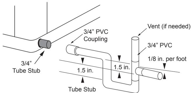
On horizontal and bottom flow units, a PVC stub or stainless steel tube is provided for condensate drain piping connection. An external trap is required (see below). If a vent is necessary, an open stand pipe may be applied to a tee in the field-installed condensate piping.
