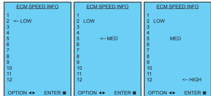
After the high speed setting is selected the AID Tool will automatically transfer back to the ECM Setup screen.
