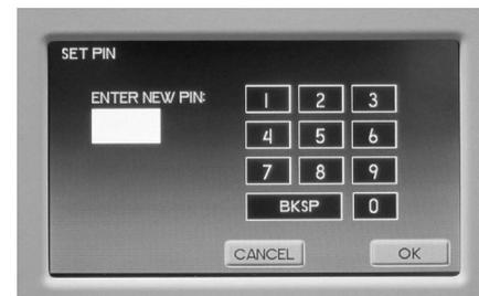
This thermostat has the option to set security features to lockout everything but the adjustment of the temperature.
