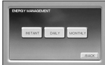
1. If your heat pump has Energy Monitoring installed, the energy consumed can be viewed by pressing the Energy button.
