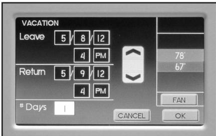
1. From the MENU, press the Vacation button to set vacation starting date, time, and desired temperature, return date, time.
