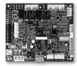
condensate (with AHB in air handler) and freeze detection, over/under voltage faults, along with communicating thermostat capability for complete fault detection text at the thermostat.
