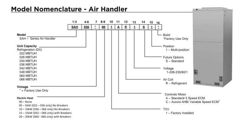
Note: To field convert the SAH to bottomflow air discharge. The SAHBCK kit must be ordered separately. Note: Air flow on the 060 and 066 units in the horizontal configurations should be limited to 1900 cfm in cooling mode, or condensate blow off may occur.
