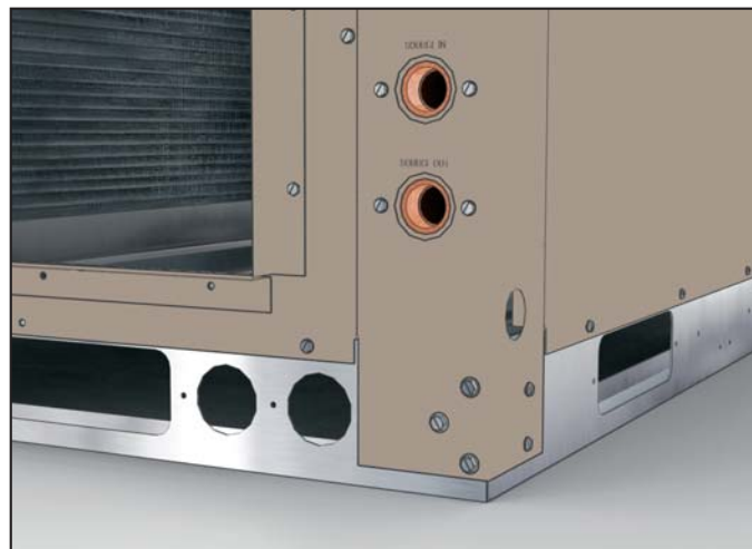
Figure 4B: Side Water Line Connections
